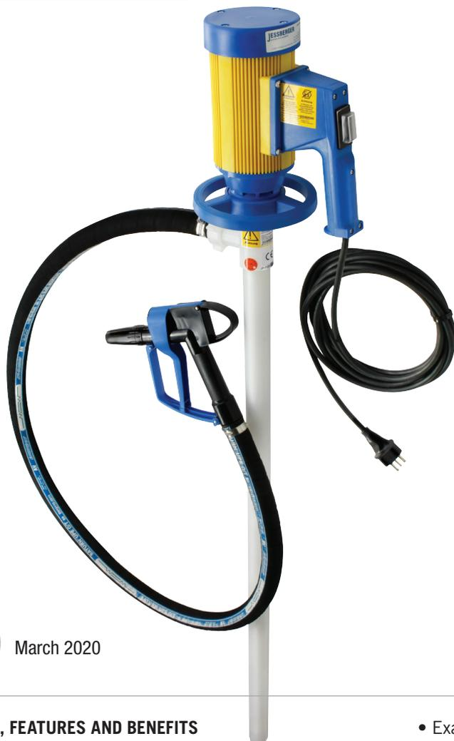
The JP-280-PVDF-HC-1000 drum pump kit with a 240V electric motor and pump tube made of Polyvinylidene fluoride is designed and manufactured in Germany. This light-weight and powerful pump is suitable for transferring and pumping small quantities of neutral or highly aggressive fluids out of 205L plastic drums.
