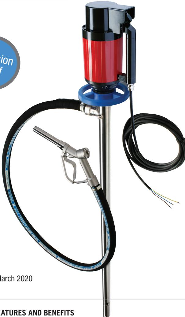
The JP-440EX-SS-SS-1000 drum pump kit with a 240V ex-proof electric motor and pump tube made of stainless steel is designed and manufactured in Germany. This light-weight and powerful pump is suitable for transferring and pumping small quantities of flammable liquids out of 205L steel drums.
