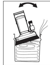
3. Snap cord and hose keepers in place in their respective slots in cabinet lip. Connect high pressure hose and grease gun.
